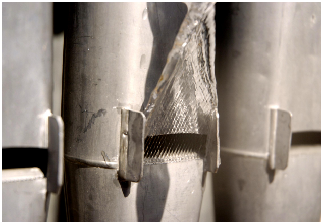
Figure 4: The waterpipe organflute: reverse modulation of a pipe organ with water flow. Increased water flow reduces the sound output of the organ pipe. The outer two pipes shown here are sounding at full volume, while the middle one is at minimum volume. Selective modulation of the organ pipes with water jets that can be touched by a user provides an immersive and direct experience.
