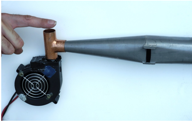
Figure 1: Basic principle of operation for direct fluid user interface: This user interface allows a person to engage the fluid directly, i.e. to manipulate the fluid that is then making the sound by way of touching it in various ways. Touching the jet of fluid forces it out through a whistle, flute, or organ pipe, while also allowing the user to feel the fluid on the hand and fingers. When not touching the jet, the fluid comes out the jet, causing the side discharge of the tee fitting to be in vacuum, by way of the Bernoulli principle of fluid flow. Thus the note is sounded when the fluid is touched, and the sound stops when the user takes his or her finger away from the output port.
