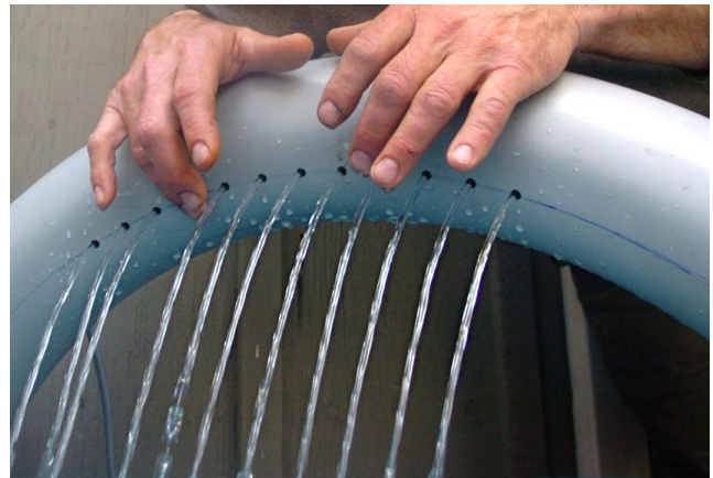
Figure 11: Making the electronic organflute resemble its acoustic counterpart: Here I have hidden the 12 restrictometers, a 12 channel analog to digital converter, and all of the computation and sound synthesis hardware inside an aesthetically pleasing housing that compliments the curved arcs that the water jets make. The picture shows the organflute being played over a hot tub, during an outdoor Mother’s Day performance, May 2005. This organflute pumps water out of the tub, and the water then lands back into the tub to be recirculated. A waterproof speaker inside the pipe makes the sound, so that the sound appears to come from the instrument, in the same way it does with an acoustic organflute.
