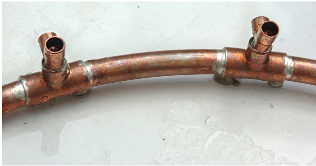
Figure 3: Fluid chest (flow chest): A manifold carries a water supply to upward jets that point up, but are angled slightly inwards towards a bather/user standing in the center of the fountain. When one or more of the upwards facing fluid jets are blocked, fluid is diverted outwards to one or more output devices that can produce sound to generate individual musical notes or chords.
