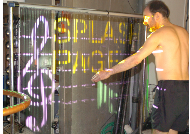
Figure 13: Put on your surf shorts to surf the web: Splashing through cyberspace... A “SPLASH PAGE” is made from a 144-note linear organflute turned upside-down and illuminated with a data projector. The system detects the location of where the hand is inserted into the “waterfall” of the splash page, so that an immersive interactive multimedia experience is possible. The green arrow under the left palm is the cursor. The curved portion of copper pipe to the left is a 61-note organflute located to the left of the splash page. It is a free-standing sculpture connected to the same water supply and computer systems as the splashpage.
