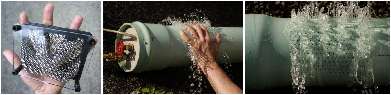
Figure 14: Invention of the splashscreen, inspired by the pinscreen: Left hand print on the metal rods of the well-known pinscreen invention. Middle and right images: A new invention of my own, inspired by the pinscreen. I call it the “splashscreen”.
