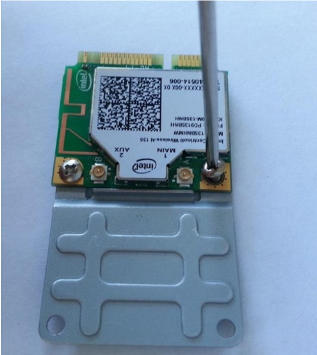
Figure 5-1. Connecting the bracket to the WiFi card
