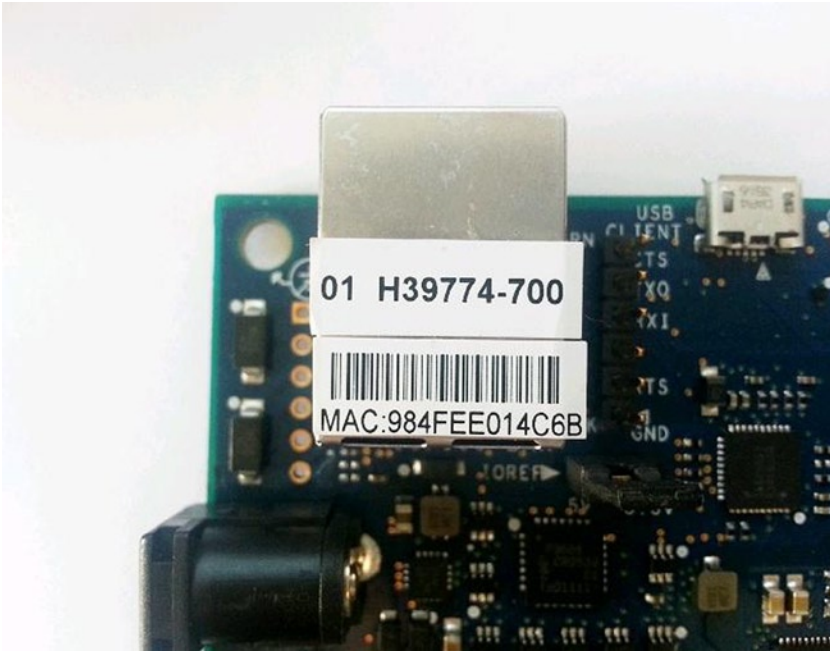
Figure 2-14. The white label with the exclusive Ethernet MAC address
